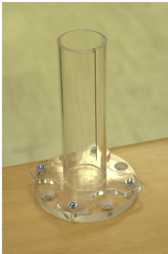
Figure 3.5: Calibration phantom for the first generation VRX-CBCT. The phantom consists of a thin lead wire mounted on the side of an acrylic tube.
