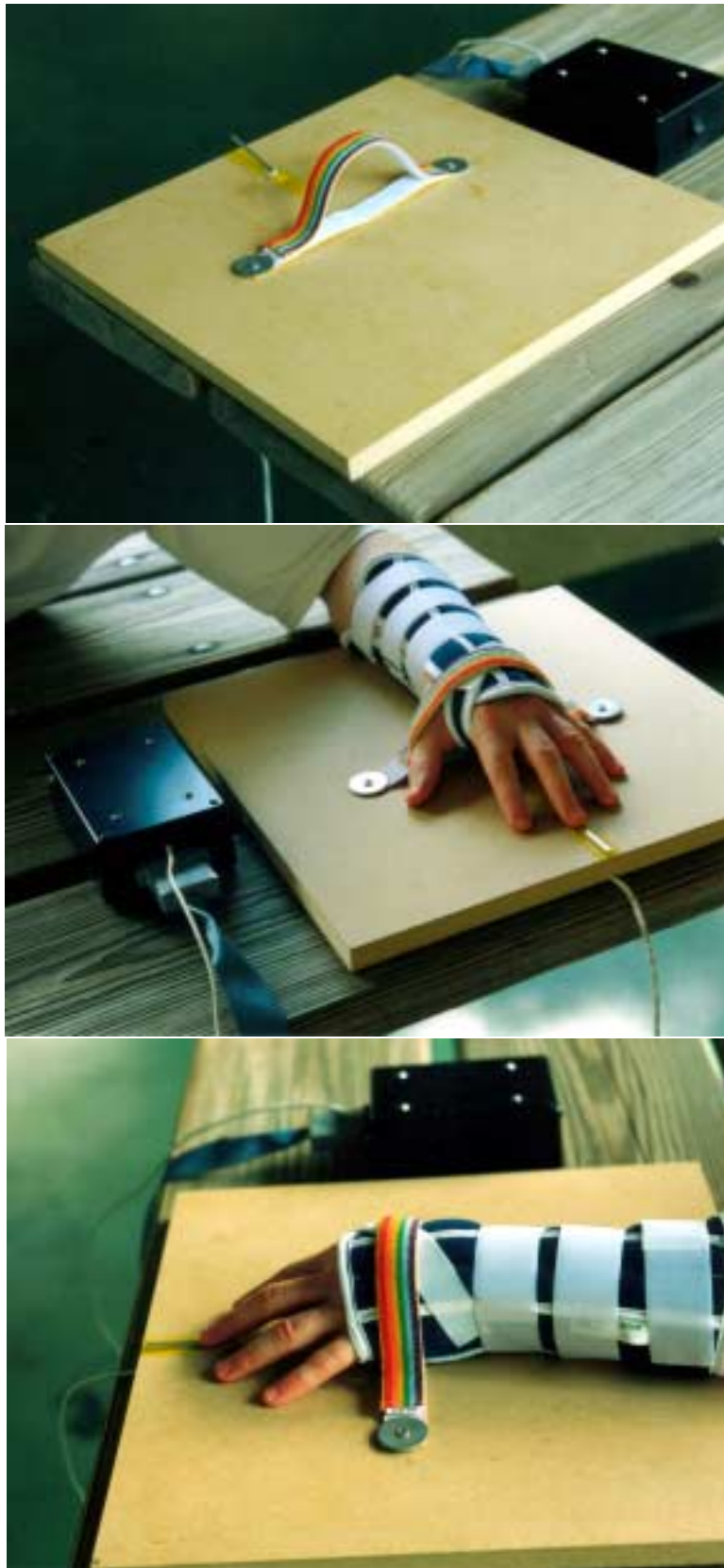
Figure 2.7. The triggering device for use in passive movement tests.
