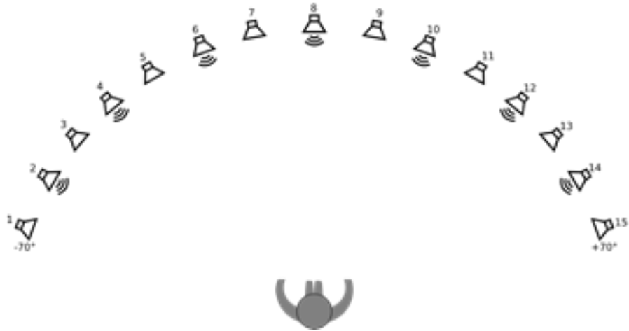
Figure 3-1. Localization speaker test set-up.
