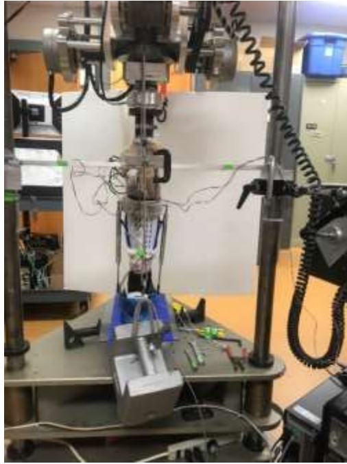
Figure B-7. Posterior View of Testing Setup Showing the Static Achilles Load for Study 2.
