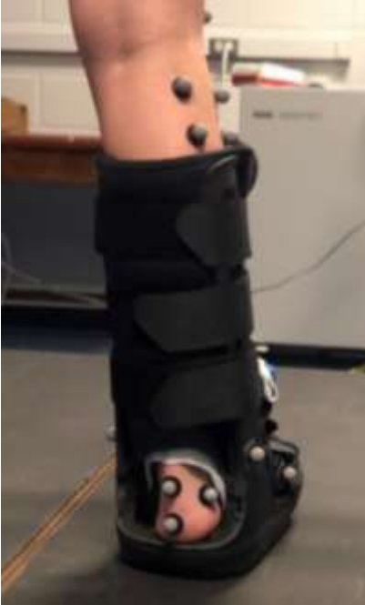
Figure 3-2. Foam Material Removed from Walking Boot to Expose the Heel to Track Foot Motion.
