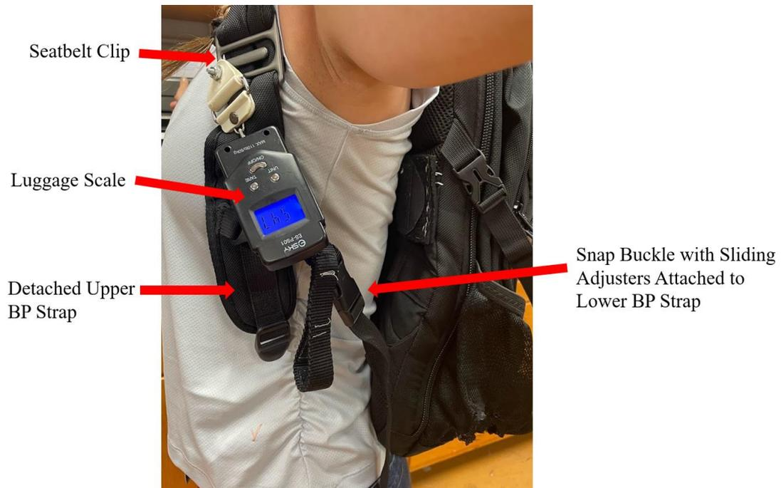
**Figure 3-7. Strap Tension Measurement Set Up.**
