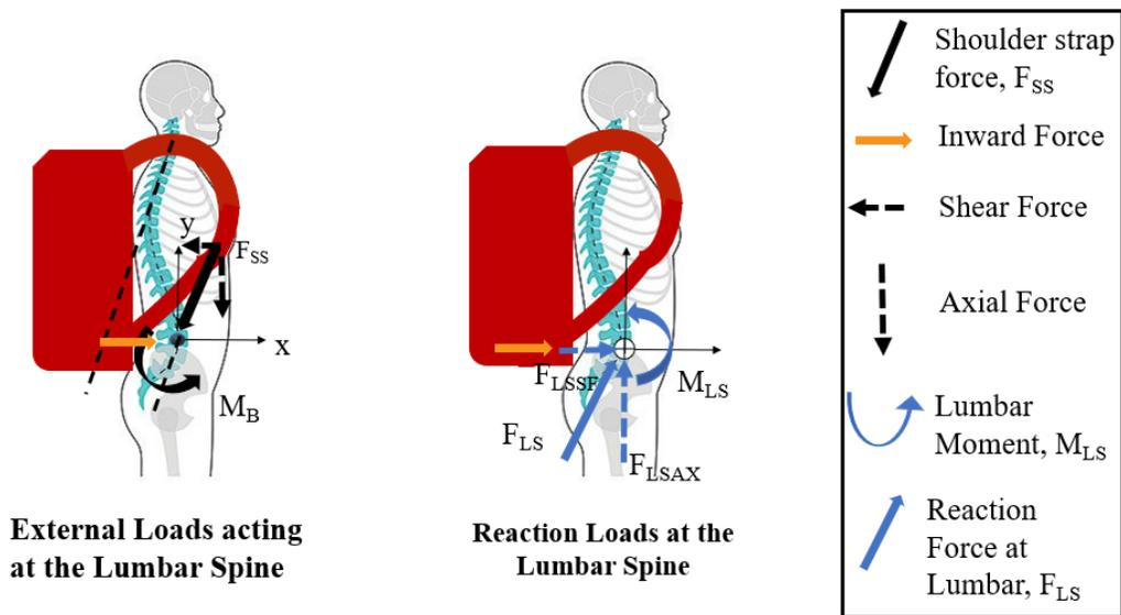
**Figure 3-1. External and Internal Spine Loads with a Backpack.**
