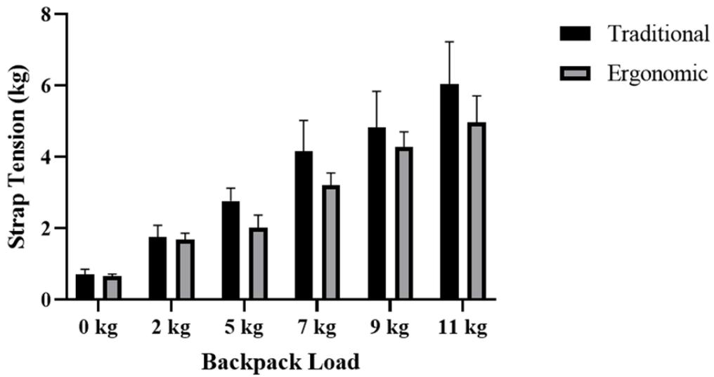
**Figure 3-9. Strap Tension Measurements in Each Backpack Condition.**
