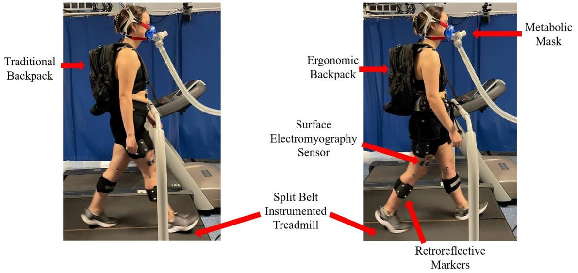
**Figure 4-7. Functional Gait Study Test Set Up.**
