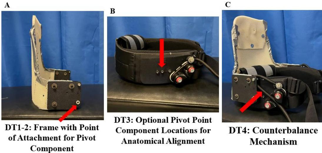
**Figure 3-6. Ergonomic Backpack Features Based on Design Tasks.**
