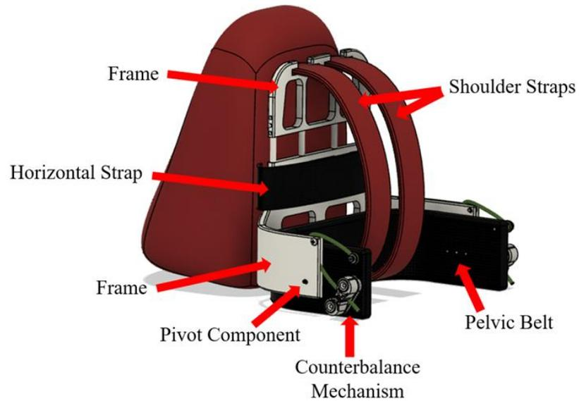
**Figure 2-11. Assembled Ergonomic Backpack Concept.**
