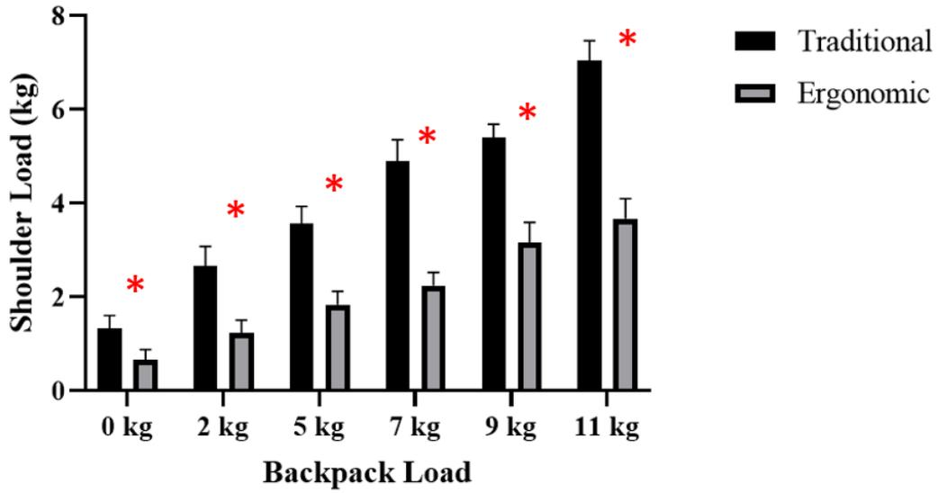
**Figure 3-10. Shoulder Load Measurements in Each Backpack Condition.**
