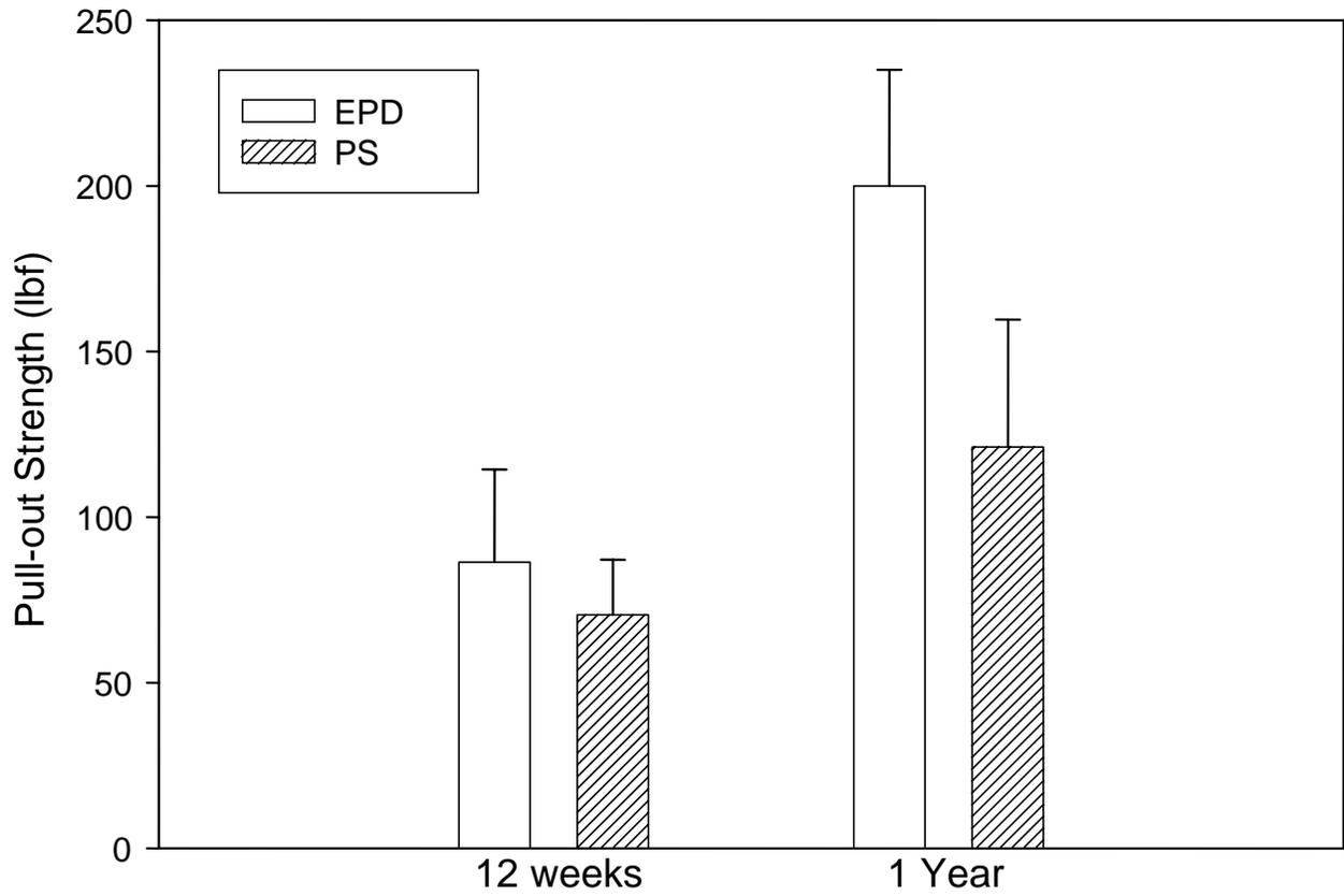
Figure 1. Mean interfacial strength with standard deviations of EPD nano HA and PS HA coated implants after 12 weeks and 1 year of implantation.
